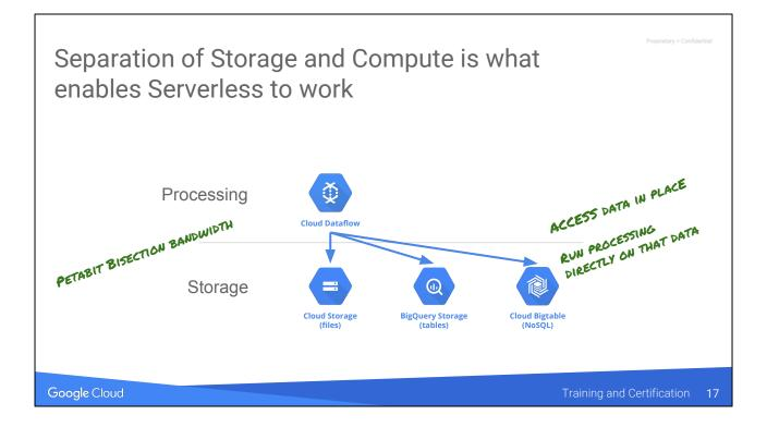
Separation of storage and compute is what enables "serverless to work" --Dataflow can read use any of these as source/sink. This sort of direct read is efficient because of very high sustained read speed from Cloud Storage -- any two computers in data center are connected by very fast network.
