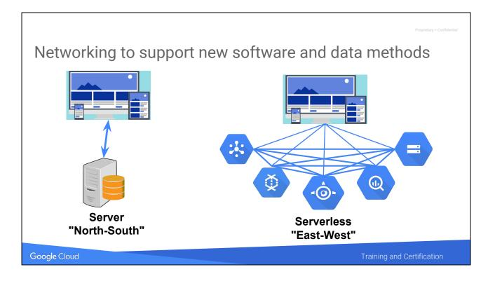
Networking within a data center used to be focused on transactions between a client and a server, what is called "North-South" communications. For example, a user might request a web page, and the server generates the web page. In that paradigm, the network needs to support low latency transactions between the user and the server.
