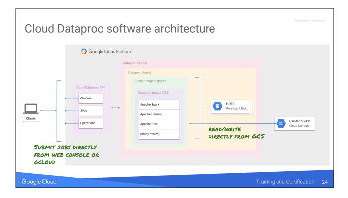
Can directly read/write to GCS from Spark, Pig, etc. Submit jobs
